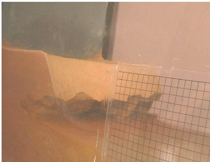
Figure 1: (a) Centrifuge paddle generated fluid waves and (b) soft cliff erosion models showing wave damage (after [17]).
