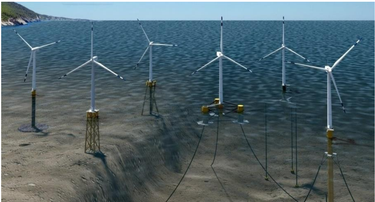
Figure 3-1 - OSW Foundation Types. From left to right: Monopile (fixed), Jacket (fixed), Twisted jacket (fixed), Semi-Submersible Platform (floating), Tension-Leg Platform (floating), and Spar-Buoy (floating) [3]
