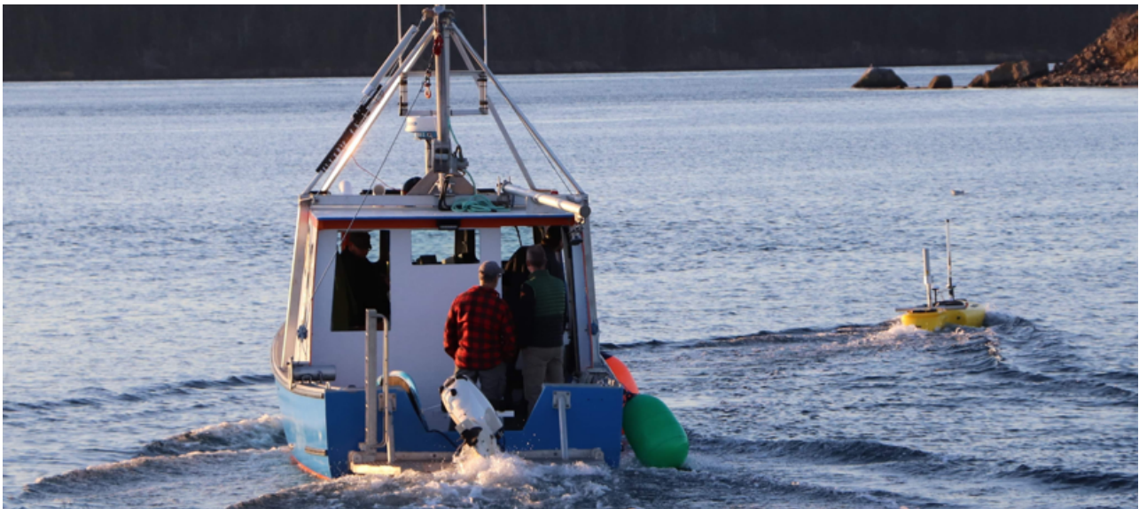
The Grand Adventure and initial system testing for the Jetyak, an autonomous jet powered kayak, carrying the Ping DSP sonar. On the boat are Richard Cheel (Dalhousie University), Dr. Alex Hay (Dalhousie University), Dr. Brian Ward (National University of Ireland Galway), and Greg Trowse (SOAR). Photo credit: Amy Tudor, freelance photographer, Westport, NS.
