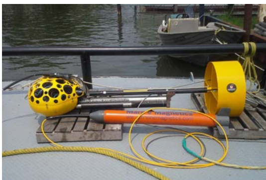
Geophysical - combined side scan sonar, chirp profiler and magnetometer.
