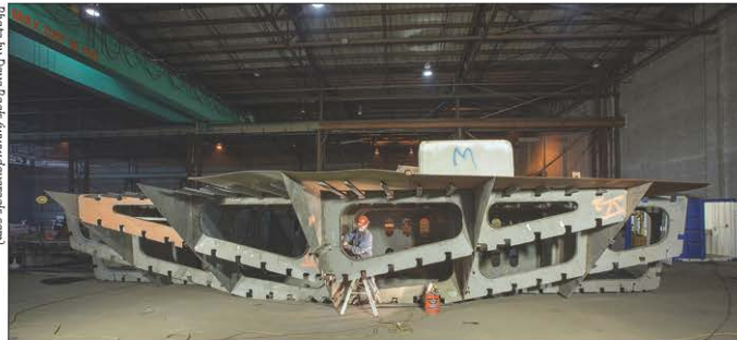
The superstructure that will house the turbine will be fitted to the hull (below).
